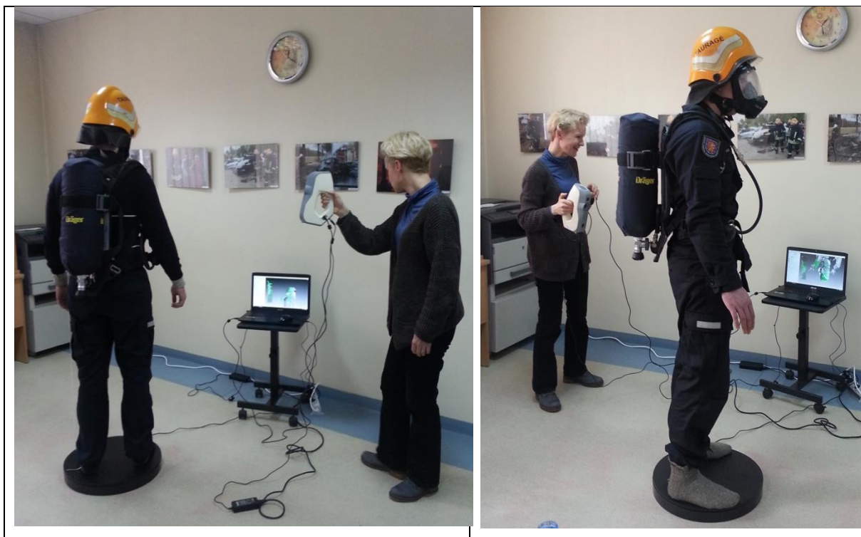
Fig. 2. Process of scanning using portable scanner
